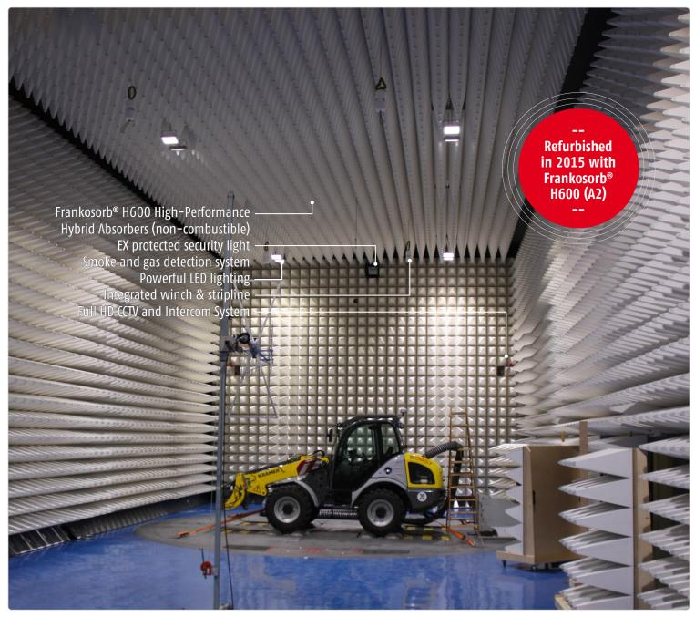
▶ This chamber built in 1998 was equipped with carbon-loaded foam absorbers and in use for about 15 years. For 5 years the absorbers drastically dried and completely lost performance. Unfortunately, the customer had to re-invest, but now in a future-proof and stable solution. In 2015, customers' choice was Frankonia with its unique Frankosorb® absorbers.
