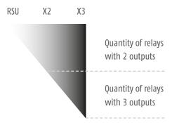
RSU 2223 = 2 relays with 2 outputs and 2 relays with 3 outputs
